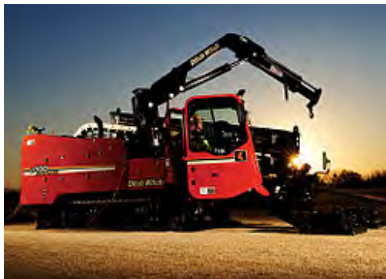
A directional boring unit in action.
